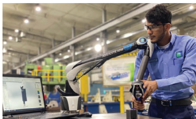
Figure 3. 3D scanning at the reverse engineering center
